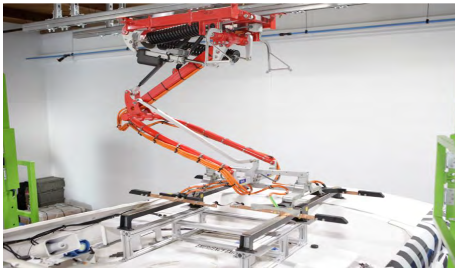
Figure 1 - Overhead Catenary/Pantograph Type Charge Head
